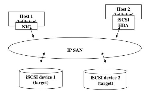
The host side needs an iSCSI initiator. The initiator is a driver which handles the SCSI traffic over iSCSI. The initiator can be software or hardware (HBA). Please refer to the certification list of iSCSI HBA(s) in Appendix A. OS native initiators or other software initiators use the standard TCP/IP stack and Ethernet hardware, while iSCSI HBA(s) use their own iSCSI and TCP/IP stacks on board.
